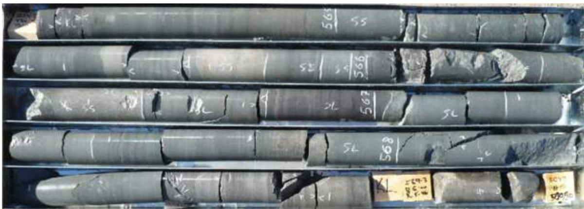
Figure 5.4 Drillcore from Paranui 10 Well showing Rewan Group Core
